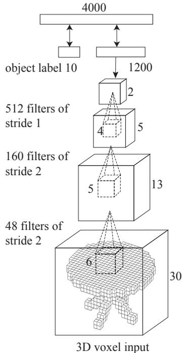
(a) Architecture of our 3D ShapeNets. For simplicity, we only show one filter for each convolutional layer.
